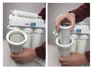
. Tighten the far left sump hand tight and secure it with the supplied filter wrench by turning it an additional 1/4 - 1/2 turn.
