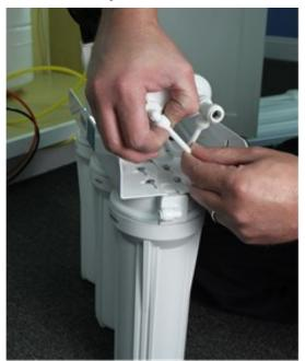
2. Use the supplied wrench to remove the membrane 4. housing cap.
