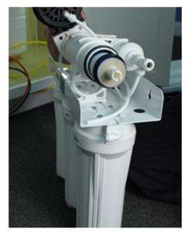
**BE SURE** the membrane is fully seated in the housing. If the membrane is fully seated, it will about 1/8 - 1/4 inset from being flush with the housing.
