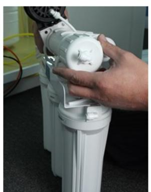
6. Push the 1/4" tubing back into the elbow fitting. **BE SURE** it is fully seated in the fitting or a leak could occur.
