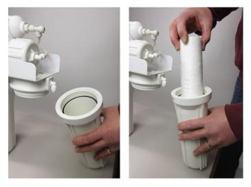
Tighten the far right sump hand tight and secure it with the supplied filter wrench by turning it an additional 1/4 - 1/2 turn.
