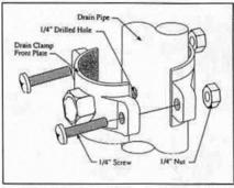
Drain saddle valve installation
