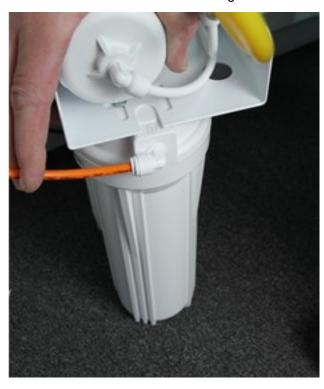
closed position. Use the supplied syringe and add 5ml of If the system is equipped with a permeate pump, clip the pump the supplied sanitizing solution to the Green tank tubing to the membrane housing using the supplied mounting bracket and make the connections to the pump using the label on the pump and the labels on the tubing. There will be a Permeate IN, Permeate OUT and Brine IN connection on the pump. The Brine OUT connection will be made in the following step.
