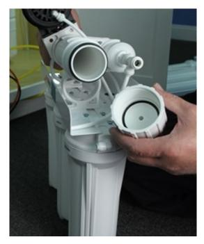
Remove the membrane from the protective packaging and install it in the membrane housing. There are two O-rings on end of the middle membrane tube. Lightly lubricate these O-rings with the supplied silicone grease.
